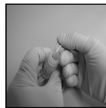
SNAP AND TWIST THE SHAFT AT THE BREAK-NOTCH TO DISLODGE LOOP INTO THE SampleTainer
